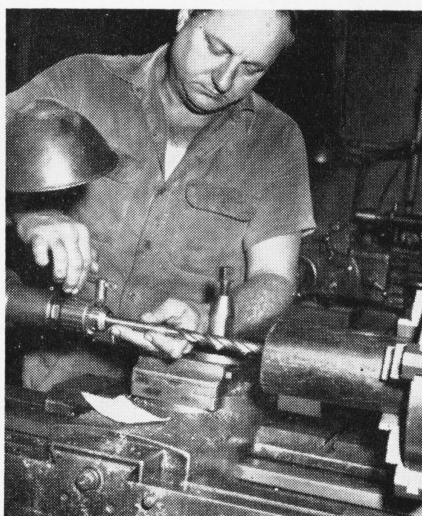
Careful Use of Tools and Materials Basil Bezuhly carefully adjusts a high-speed drill (cost $6.) into lathe before drilling into steel bar stock.
